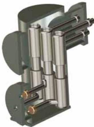
50 Hz gas-insulated switch
