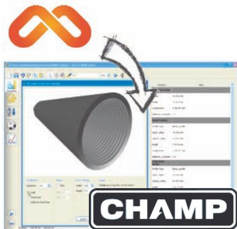
Antenna Magus now supports a third CEM analysis tool - CHAMP, a dedicated analysis tool for corrugated and smooth-walled horns with circular cross section, developed by TICRA. It is now available as an export option (along with CST Microwave Studio and FEKO) when exporting models for corrugated horn antennas.
