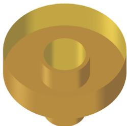
Although this is not a user requested antenna we decided to include it due to its usefulness when needing a feed for a prime focus reflector antenna with small focal-length to diameter (F/D) ratio.
