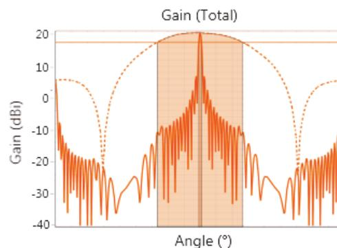
Figure 1. Gain pattern for a 20 dB Linear resonant waveguide slot.
