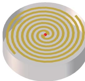
Compared to the *Cavity-backed log spiral* this antenna has similar performance characteristics but may be easier to feed and manufacture. Impedance performance of the *Cavity-backed Archimedes spiral* antenna may be slightly more erratic than the equivalent *Cavity-backed log spiral* across the band.
