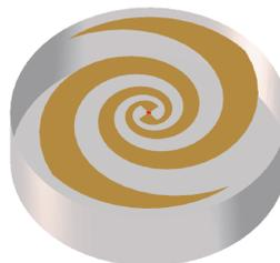
Cavity back spiral antennas have been requested by a number of Antenna Magus users.
