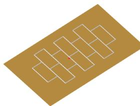
The wire-grid array was first described by Kraus back in the 1960's as a "*Backward Angle-Fire Array Antenna*" consisting of a grid situated parallel and close to a flat conducting sheet or ground plane. When fed at the
