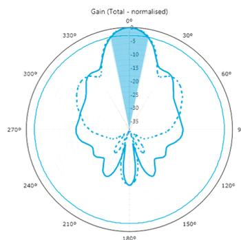
Normalised gain of the *Waveguide-fed short backfire*.
