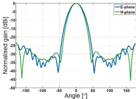
Principal plane gain patterns for the *Diagonal horn antenna*.
