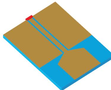
The *Trapizoidal CPW-fed monopole* is a popular ultra-wideband (UWB) antenna used in the FCC 3.1 - 10.6 GHz radio band. Due to its reduced size and wide impedance bandwidth, these printed monopoles are also popular in mobile communications.
