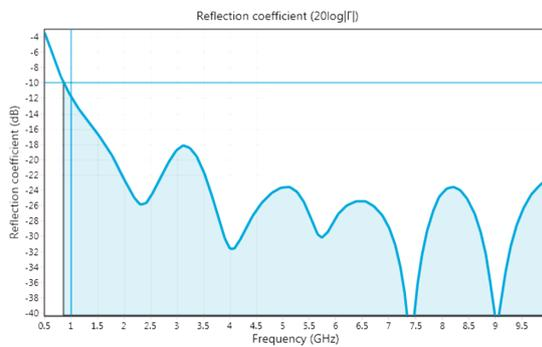
Reflection coefficient of the *Classical monocone* designed with  $F_{min} = 1\text{GHz}$ .
