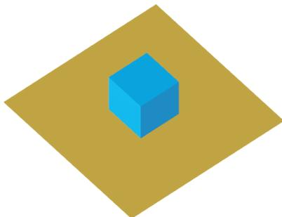
In 1983, M.W. McAllister showed that dielectric slab placed on a ground plane and excited by a pin or probe fed through the ground plane into the dielectric will radiate at its resonant frequency.
