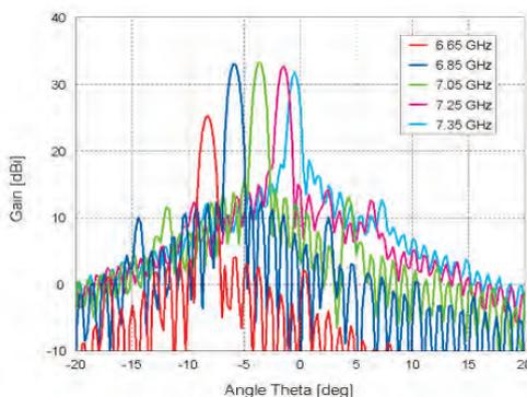
*Traveling wave slotted guide array* squint angle pattern shift vs frequency.
