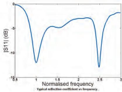
Typical S11 impedance of the *Printed dual band double T monopole*.
