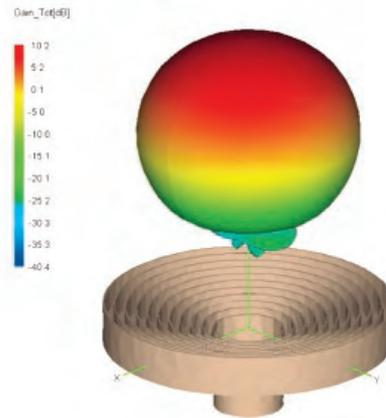
*Axial-choke* with typical 3D radiation pattern.
