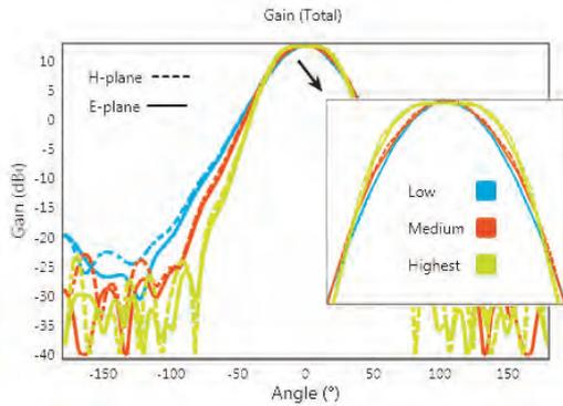
*Axial-choke* pattern cuts for three different main beam designs.
