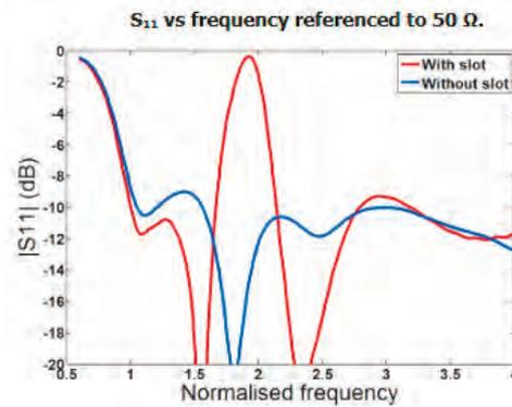
S11 comparison of the *CPW-fed trapezoidal monopole* (no slot) and the *CPW-fed notched trapezoidal monopole* (with slot).
