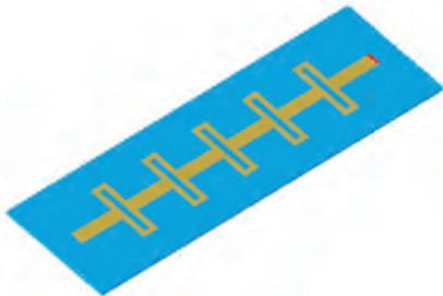
The *Microstrip Franklin array* effectively consists of thin rectangular half-wavelength patches which are connected with non-radiating, phase reversing phasing lines. The phasing lines are narrow half-wavelength microstrip lines folded into quarter-wave stubs so that the counteracting standing wave currents do not radiate. The natural current distribution is thus converted into a co-phased distribution of currents which produce only one major radiation pattern.
