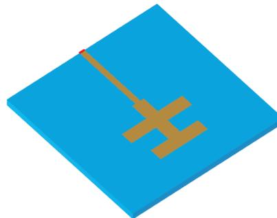
This antenna is a variation of a basic planar monopole antenna. An additional section is attached to excite a second resonance at a higher frequency. As with several other planar antennas, this monopole can be integrated on the same substrate as other electronics. The *T-shape monopole* makes the antenna more compact than a straight monopole.
