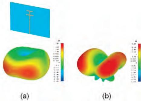
Typical gain pattern at (a) lower frequency and (b) upper frequency.
