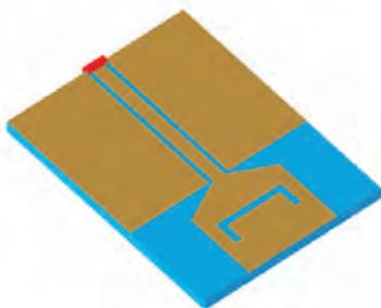
The *Notched trapezoidal monopole* is an alternative version of the *CPW-fed monopole* which was included in the database for the release of Version 1.6.0. These antennas are popular for ultra-wideband (UWB) applications (especially in the FCC 3.1 - 10.6 GHz radio band) due to the reduced size and wide impedance bandwidth that can be achieved. The addition of the slot in the monopole adds a narrow-band, high-
