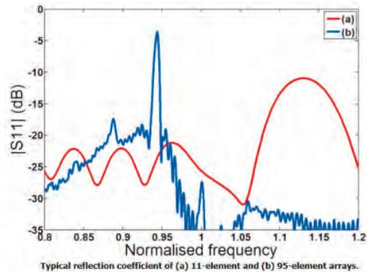
Typical  $S_{11}$  for (a) 11-element and (b) 95 element arrays
