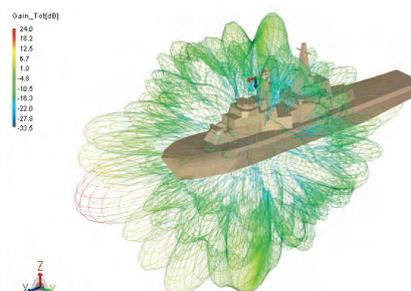
Array point source placed on a ship.
