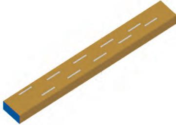
Compared to the *Resonant waveguide slot array* that is already available in Magus, the *Traveling wave slotted guide array* has some impressive advantages. It can handle higher power and operates over a much wider band (up to 25% bandwidth), where the resonant array suffers from a decreasing bandwidth as the number of elements (and hence gain) increases, whilst this array does not.
