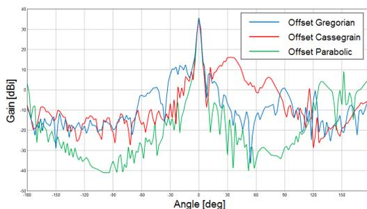
Gregorian vs Cassegrain vs Parabolic offset-fed reflector gain comparison.
