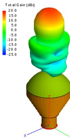
Lens horn 18 dBi gain pattern.
