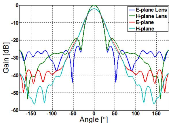
Gain comparison between an axial choke horn with and without a lens.
