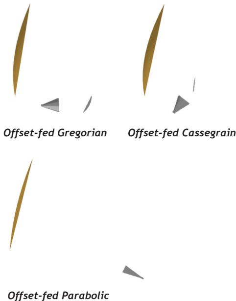
The Horn-fed offset- Gregorian and Cassegrain reflector antennas compared to an offset-fed single-reflector antenna. [Note the difference in feed-horn orientation and sub-reflector placement and the compactness of the dual reflector topologies when compared to the single reflector structure.]
