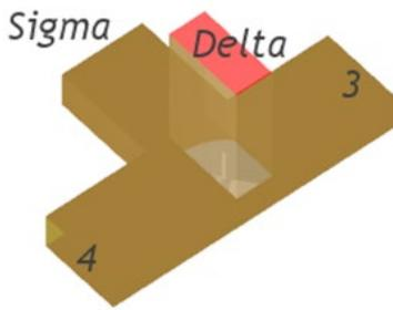
The *Magic-T* is a popular hybrid or 3 dB splitter/coupler used in many microwave systems. It was originally developed during World-War II and typically used in pulsed radar applications. One advantage of the *Magic-T* is when combining multiple power amplifiers, the input or output ports are well isolated from each other.
