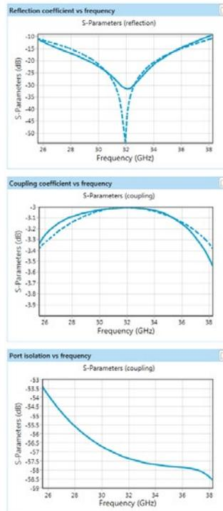
*Estimated |S11| performance showing reflection, coupling and isolation between ports for a Magic-T operating at Ka-Band.*
