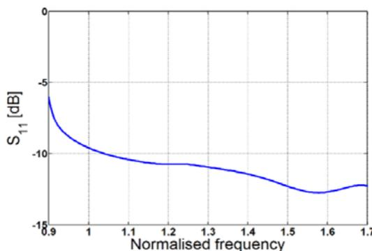
Typical reflection coefficient versus frequency.
