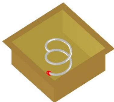
The requirement for a broadband elliptically-polarised antenna which can be flush-mounted on high speed aircraft is common in the aerospace industry. This antenna inherently fulfils the broadband, elliptical polarisation requirements. It is also mechanically simple, can be flush-mounted and is relatively small compared to other antennas that could provide similar operation at a given frequency.
