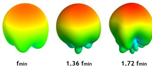
Typical circularly polarised gain patterns at the minimum, centre and maximum frequencies.
