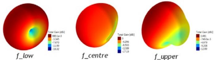
*Reflection coefficient and radiation pattern performance of a design for the GSM and IEEE802.11 bands.*
