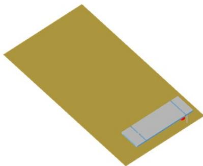
*Tri-band planar folded inverted-F antenna.*
