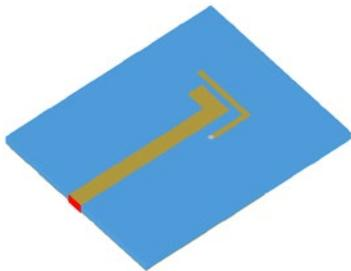
*Planar monopole with parasitic inverted L antenna*
