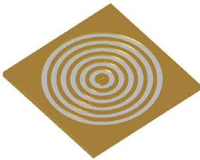
This interesting reflector feed antenna originated from optical studies which showed that sub-wavelength apertures in corrugated metallic films enhance transmission. By scaling the same concept to microwave frequencies, a very-low profile feeder antenna with approximately 20 dBi gain can be realized.
