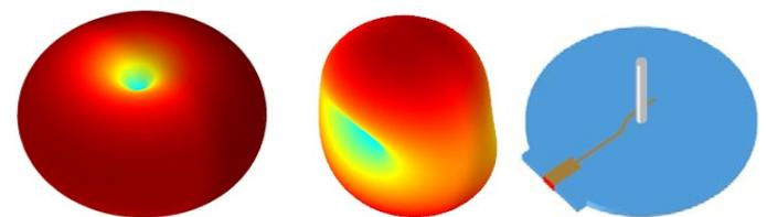
*Example: Wire monopole with annular-slot antenna for WLAN composed of quasi-omnidirectional radiators. This allows for pattern diversity capabilities.*
