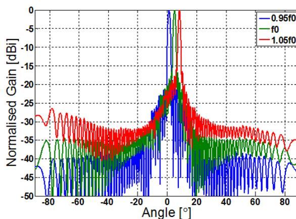
Typical main beam scan versus frequency for a 54-element array.
