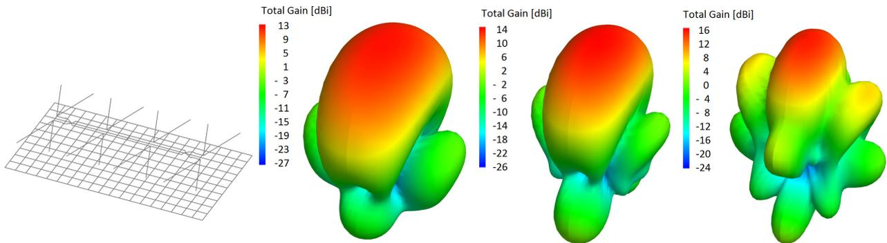
Typical 3D gain patterns at 80% of the centre frequency, at the centre frequency and at 120% of the centre frequency.
