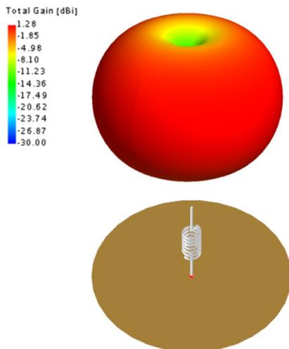
*Radiation pattern of the inductively loaded monopole illustrating the familiar omnidirectional pattern of a conventional monopole.*
