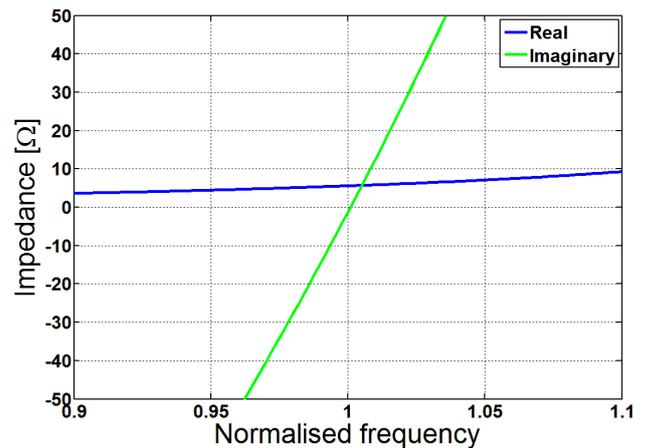
*The inductively loaded monopole antenna has a very low input impedance.*
