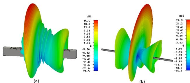
Fan-beam radiation patterns of linear traveling-wave narrow wall slotted guide arrays at the centre frequency of the operating band for (a) 12-element (with negative squint) and (b) 54-element (with positive squint) arrays.
