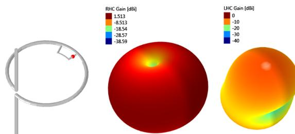
Polarisation-specific radiation patterns for a right hand circular (RHC) design.
