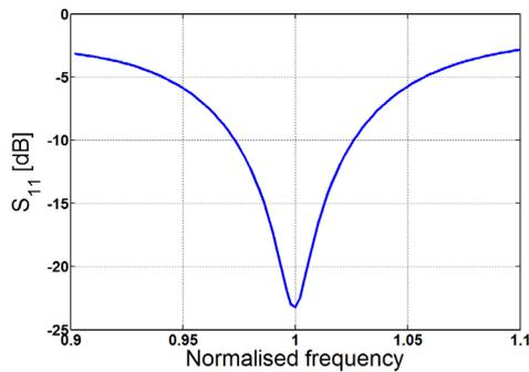
*The low-profile corrugated feeder antenna has a narrow impedance bandwidth*
