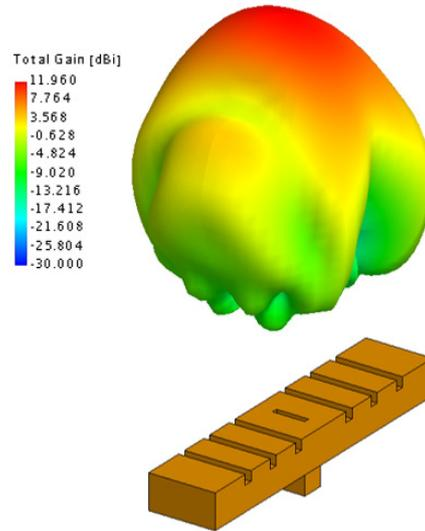
*Radiation pattern of the low-profile corrugated feeder showing medium broadside gain*
