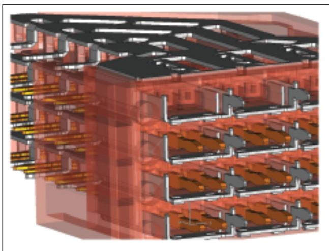
▲ Fig. 2 An ERNI Ermet zeroXT connector simulated by AdMOS. SPICE models were extracted from the full 3D broadband simulation and used in circuit simulation.
