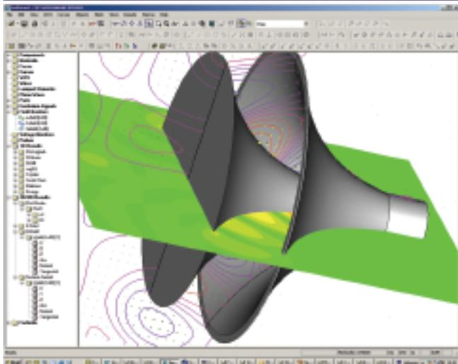
▲ Fig. 1 A coaxial horn antenna quickly constructed using the CST MWS graphical user interface.
