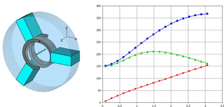
**Figure 6:** Dispersion diagram for forward mode (red), backward mode (green) and third mode (blue). The x-axis shows phase shift for one helix length. The y-axis is angular frequency.
