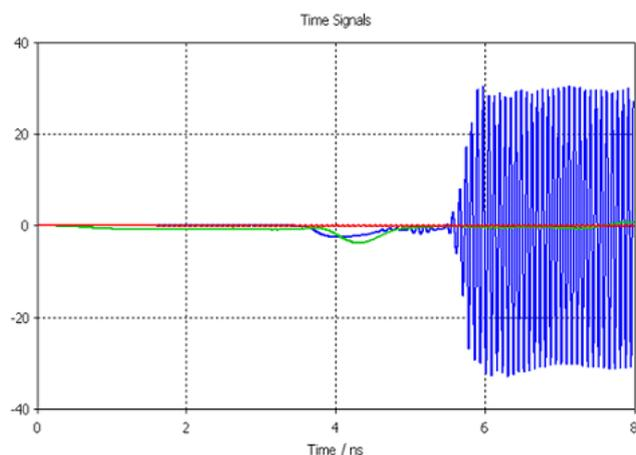
**Figure 8:** PIC simulation time signals: RF input (red), reflection (green), RF output (blue)
