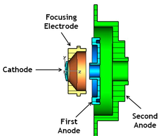
**Figure 2:** Structure of the electron gun.
