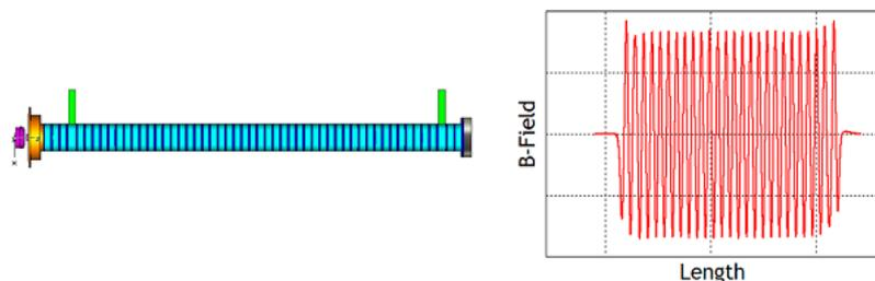
**Figure 5:** Periodic Permanent Magnet (PPM) structure (left) and resulting longitudinal magnetostatic field along longitudinal axis (right)
