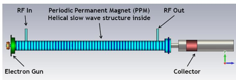
**Figure 1:** Traveling Wave Tube Structure
